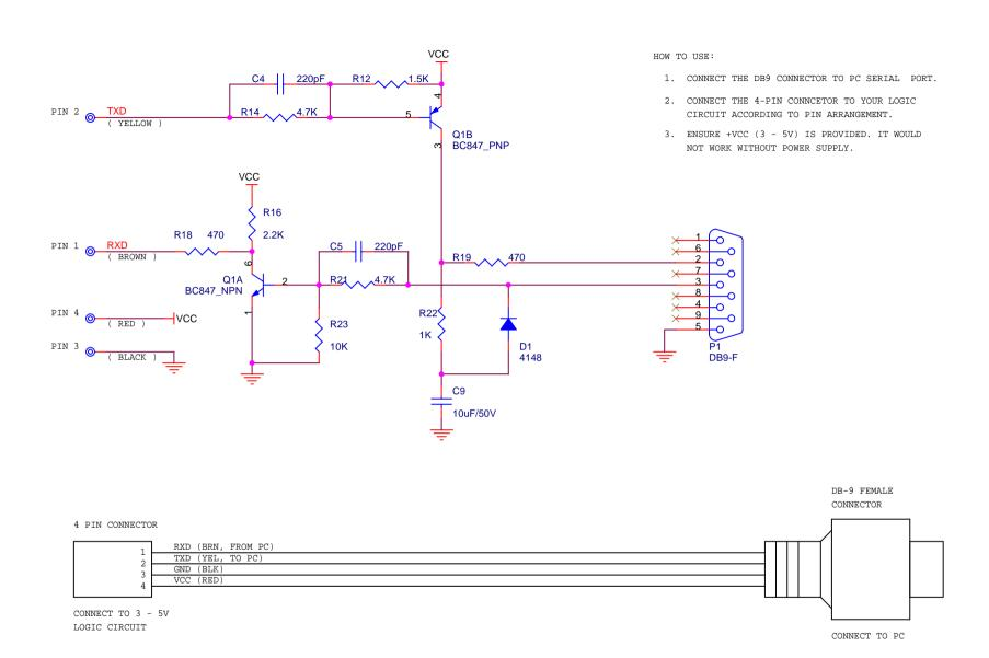
Serial Port Level Converter - WWW.JYETECH.COM
