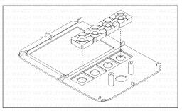
Align and press the LCD screen onto the screen panel. Fold over the PCB carefully to cover the LCD screen.
