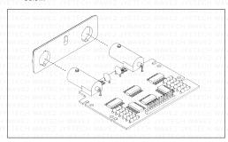
Insert the assembled Analog Board onto the Back Enclosure Panel and secure the board using four M2x4 screws.
