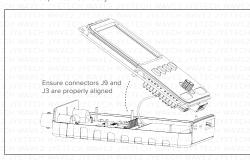
Finally, place the Top Cover and secure it using four M2x6 screws. Attach the Dial over the Rotary Encoder to complete the assembly.
