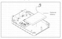
4 Slide the Bottom Cover into the Back Enclosure, ensuring the micro-USB and Auxiliary Port are positioned as shown in the following diagram:
