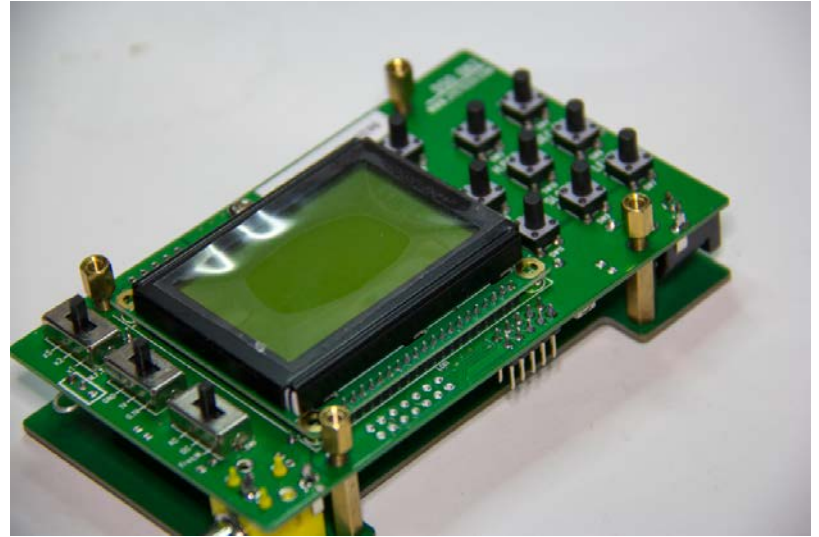
Figure 5.3-1: Start assembly from the back plate and 4 long standoffs
