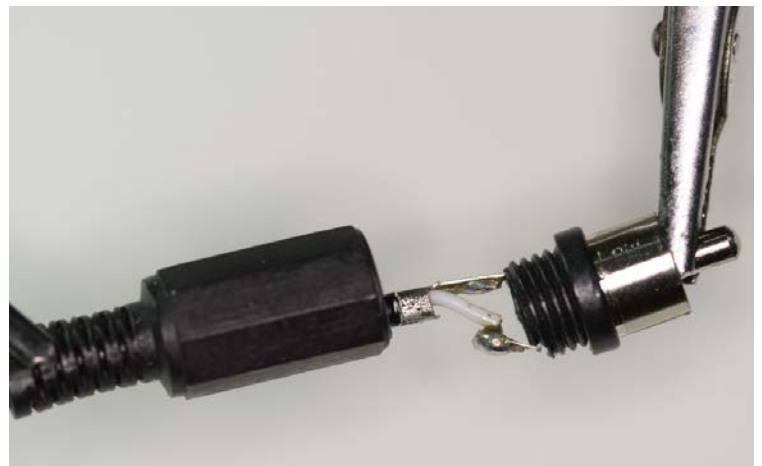
Figure 6.1-1: Probe cable assembly details
